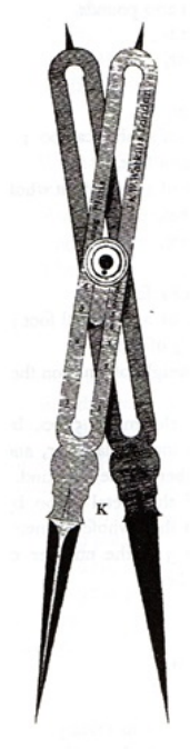
Figura 6: proportional compass [Barrow, 1792].
